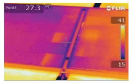
Hot spots are areas of elevated temperature affecting only part of the solar panel. They are a result of a localised decrease in efficiency, which results in lower power output and an acceleration of material degradation in the affected area.
